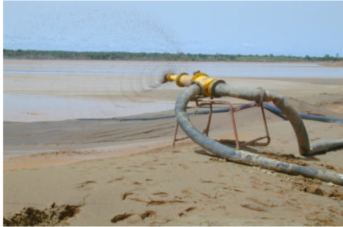
Figure 5: Sadiola deposit showing narrow sand beach – note overflow discharge location to ‘pond’ at end of short beach
